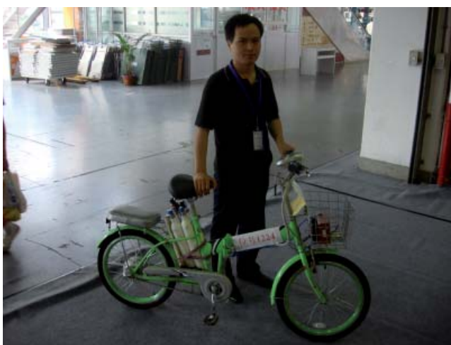
Mr. Dong Hui, Vice President of Shanghai Pearl Hydrogen Power Source Technology Company Ltd., demonstrating his company's metal-hydride powered PEM bicycle.
